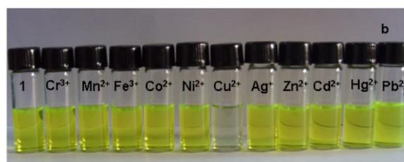
Fig. 1. (a) Absorption spectra change of **1** (20  $\mu\text{M}$ ) upon addition of different metal cations (5 equiv.) in an acetonitrile/water mixed solvents (8:2, v/v). (b) Color change of **1** in the presence of various metal cations. (For interpretation of the references to color in this figure legend, the reader is referred to the web version of this paper.)
