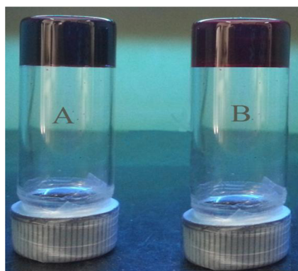
Fig. 13 Photographs of the gel of trimer 1 (a) in THF/methanol (4/1) and trimer 2 (b) in MCH
